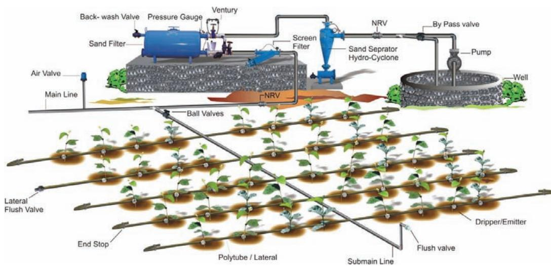
**Figure 2-5. Model Design of JISL's Drip Irrigation System**
