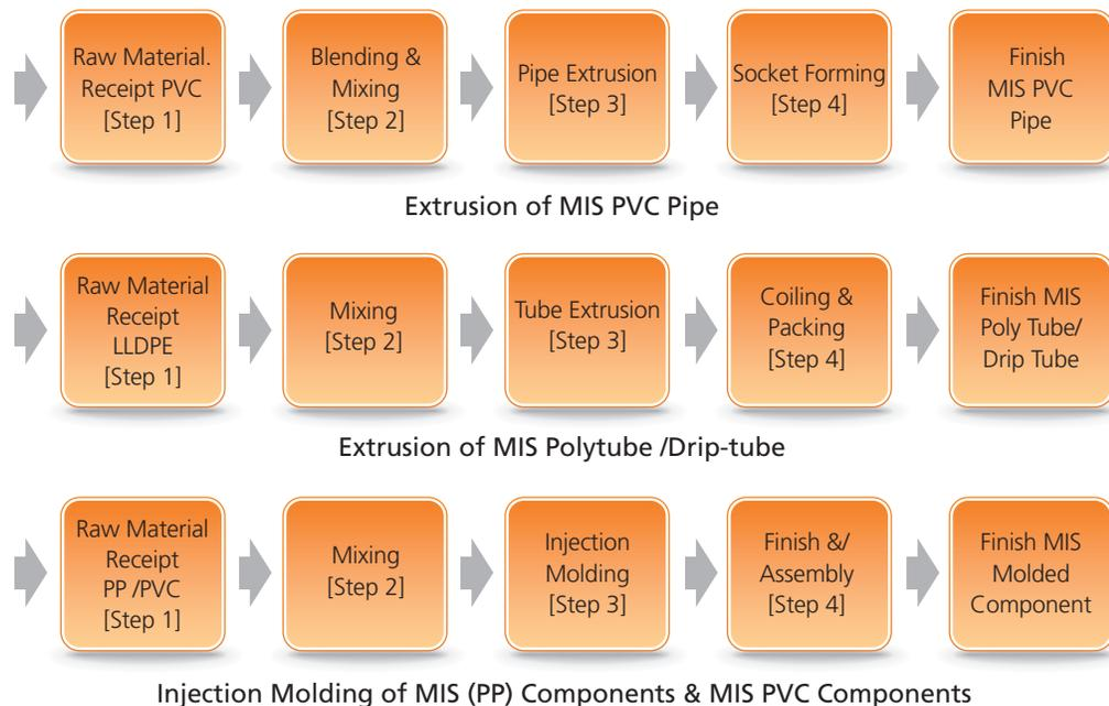
**Figure 2-6. Process Diagrams for MIS Components**
